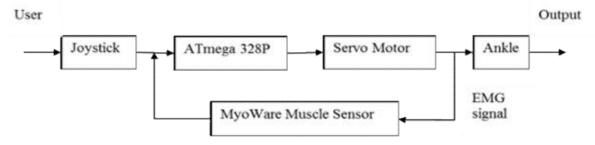
Fig.1. Block diagram of the device
