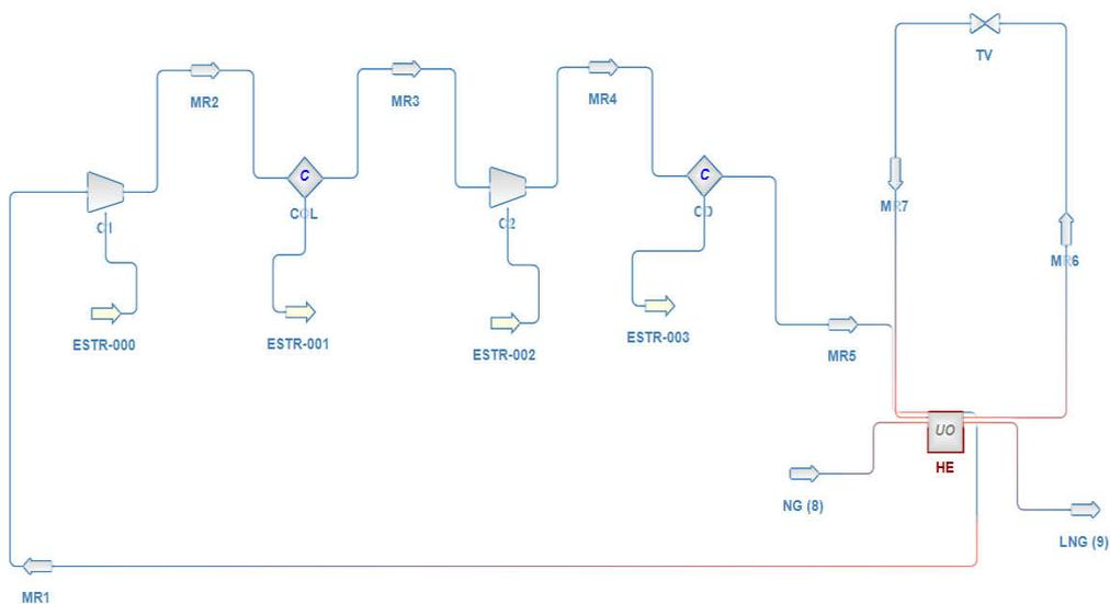
Fig.A2. Flowsheet of PRICO process as simulated in DWSIM
