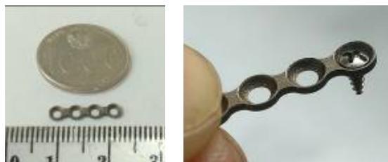
**Fig.4.** The fabrication result of miniplate prototype
