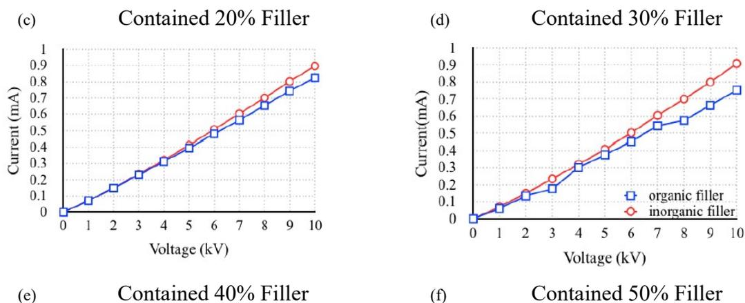
**Fig.2.** Comparison between the I-V characteristic of RTV using organic filler and inorganic filler in the same ratio
