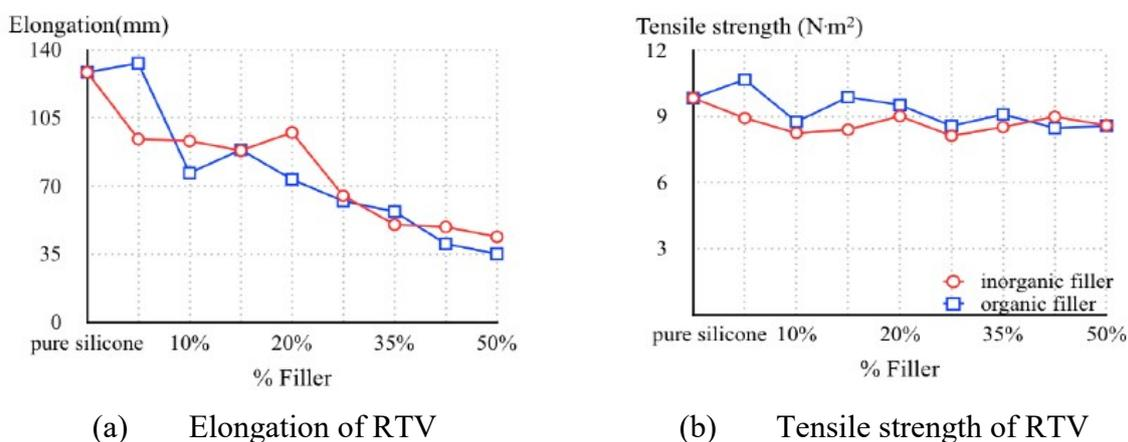
**Fig.3.** Comparison of (a) elongation (b) Tensile strength of RTV with organic and inorganic filler
