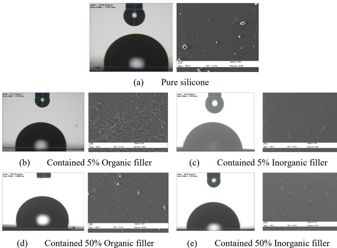
Fig.5. Image sequences of water droplets (5µL) of RTV's surface using organic and inorganic filler (Left) and Image of RTV's surface using scanning electron microscope (SEMs) (Right)
