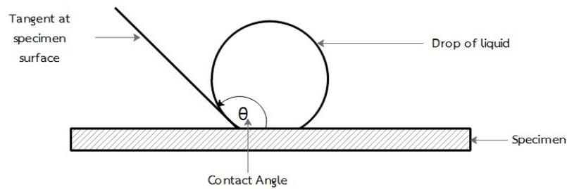
**Fig.1.** Measuring angle of contact
