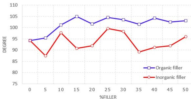
Fig.4. Contact angle of RTV with organic and inorganic filler
