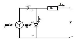
Fig.4. Equivalent circuit of wind turbine
