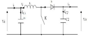
Fig.8. Equivalent Circuit of a Boost Converter
