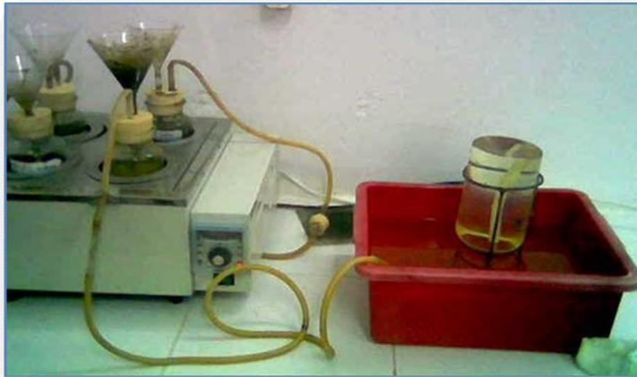
**Fig.4.** Adopted system of quantification of experimental biogas
