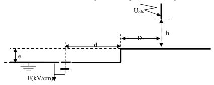
Fig. IV.3. Second configuration: Experimental arrangement for electric field measurement discontinuous earth.
