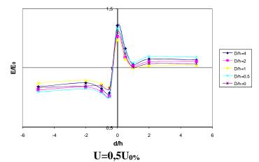
Fig. IV.4. Electric field on the ground according to the position (d/h) of the probe h=12cm
