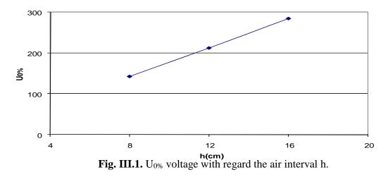
We consider  $U_{0\%}$  as being the voltage having a probability of discharge equal to 0.1% on the Gausso-arithmetic scale.
