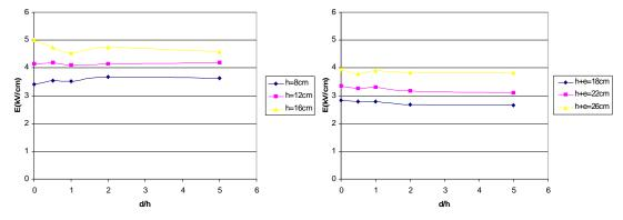
**Fig.IV.1.** Electric field measured on the earth according to the position d/h of the probe (Voltage level U = 0.5U0%)
