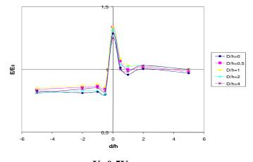
$U=0,5U_{0\%}$ Fig.IV.4. Electric field on the ground according to the position (d/h) of the probe h=12cm
