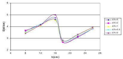
Fig.IV.1. Electric field measured on the earth according to the h of the probe
