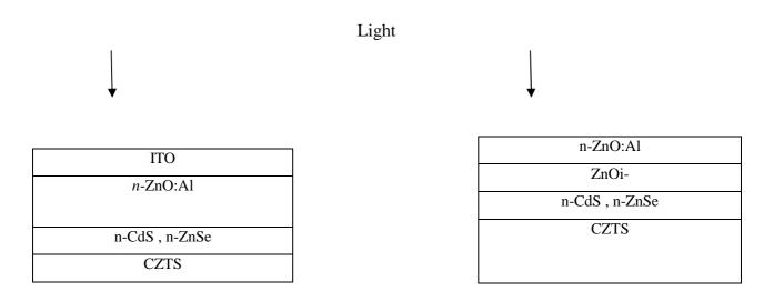
Fig.2. Structure of Solar cell
