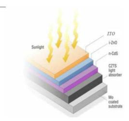
Fig.1. Structure of a photovoltaic cell CZTS
