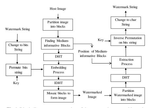
Fig.1. Block diagram representation of the proposed watermarking scheme.
