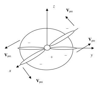
Fig. 4. The photon's cross section at  $\check{S}t' = 2f n$ . The positive charge near the axis OZ is indicated with +, the negative charges of the lobes are indicated with -.
