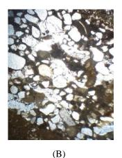
(A) (B) **Fig.9.** Microscopic photography: (A) RCC with PP fiber, (B) RCC without PP fiber
