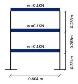
Fig.4.18. two dimensions Frame
