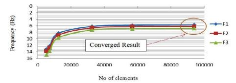
Fig.4.12. Convergence study of experimental model
