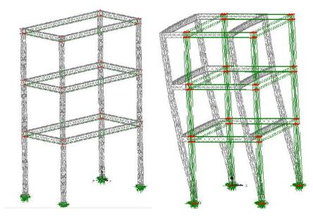
**Fig.4.15.** Unreformed and Deformed Shape of Small 1:15 Models Under Self-Weight In Eigenvalue Analysis
