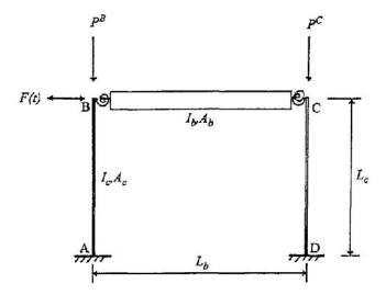
Fig.4.21. Parametric Description of Semirigid Frame
