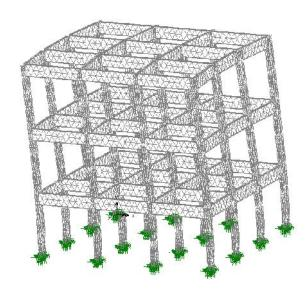
Fig.4.14. Deformed shape of Rigid Connection Steel Frame
