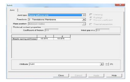
**Fig.4.9.** Joint stiffness settings in semi rigid frames
