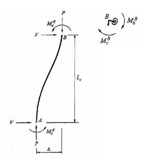
Fig.4.22. Free body diagrams of columns and joints
