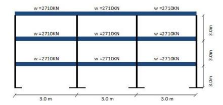
Fig.4.19. Three story-three span Steel frame as modeled in LUSAS
