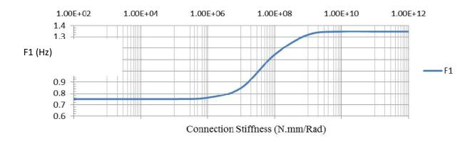
Fig.4.23. Connection Stiffness and Fundamental frequencies Using Equation 4.4
