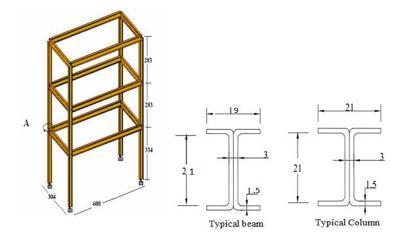
Fig.4.10. Dimensions and Details of 1:15 model
