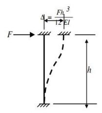
Fig.4.17. Flexural Deformation of column between rigid beams
