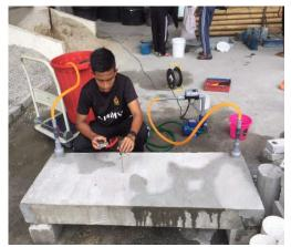
c) Tested of temperature of slab with water flowing inside the panel
