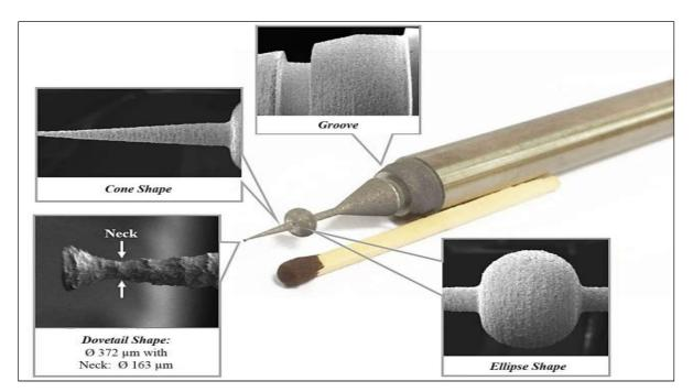
Fig.8. Different geometries for evaluating machining capability
