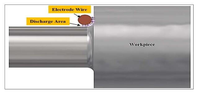
Fig.6. The phenomena discharge area in HWEDT along the electrode wire
