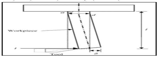
Fig.4. Workpiece deflection in the micro turning process
