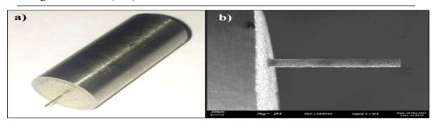
**Fig.7.** A 250 μm straight cylindrical part fabricated by HWEDT (a) actual part (b) SEM micrograph
