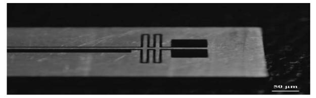
Fig.3. Image of a micro actuator [15]
