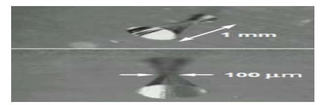
Fig.2. Image of a micro valve with a throat diameter of  $100 \ \mu m$  [14]
