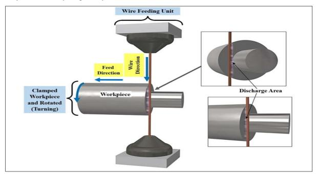
Fig.5. The HWEDT working principle
