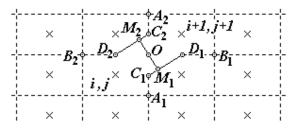
Fig.1. Modification of cells in the case when the runoff is directed along the diagonal from the cell  $D_{i,j}$  to the cell  $D_{i+1,j}$
