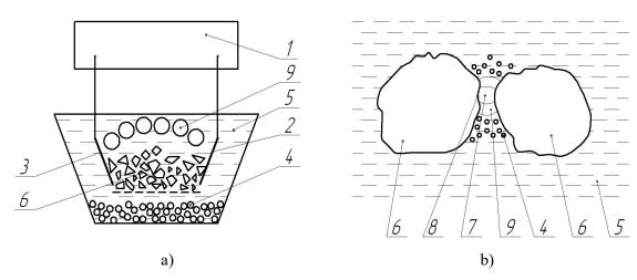
Fig.1. EED process: a) device scheme; b) process scheme
