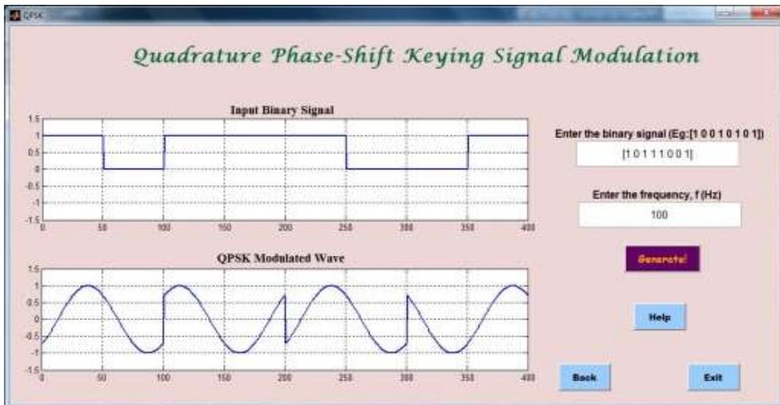
Fig.15. Quadrature phase-shift keying signal modulation
