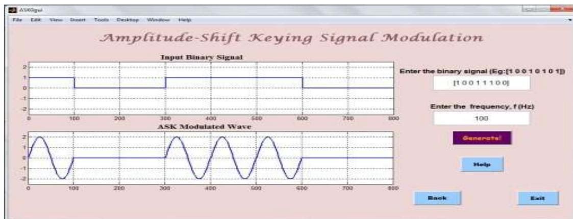
Fig.14. Amplitude-shift keying signal modulation
