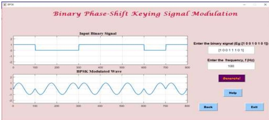
Fig.16. Binary phase-shift keying signal modulation
