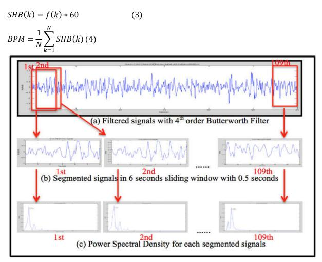
Fig.45. The procedures to extract heart beat rate through video imaging technique
