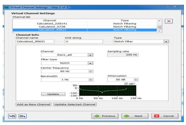
Fig.8. Virtual channel setting in NI-LabVIEW ECG feature extractor to filter power line interference
