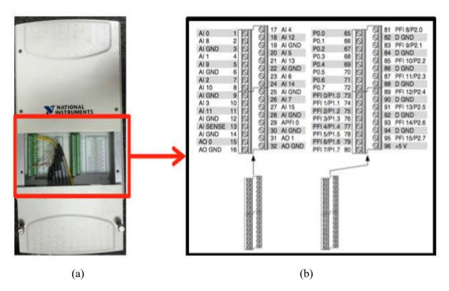
Fig.6. (a) NI USB-6281 DAQ device. (b) NI USB-6281 labelled screw terminal pinout[27]
