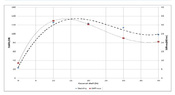
Fig.2. Stability and stiffness versus coconut shell
