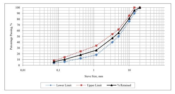
**Fig.1.**Gradation limit for asphaltic concrete [14]
