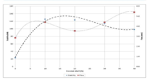
Fig.3. Stability and flowversus coconut shell
