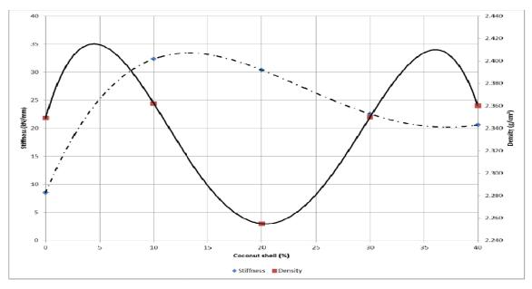
Fig.5. Stiffness and density versus coconut shell
