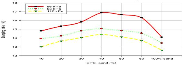
Fig.7. Damping ratio of EPS-sand mixtures and control sand sample
