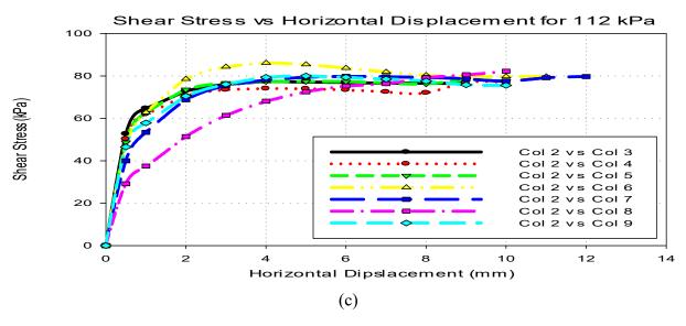
Fig.6. Shear stress versus horizontal displacement graph of (a) 56 kPa (b) 83 kPa (c) 112 kPa Damping Ratio vs EPS- sand Percentage
