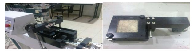
Fig.2. Shear box test for EPS-sand mixture
