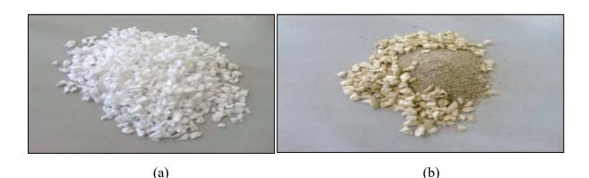
Fig.1.Samples of (a) raw shredded EPS (b) EPSsand mixture
