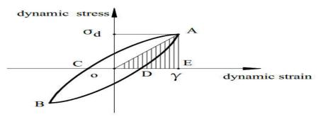
Fig.4. Dynamic stress and strain for damping ratio [13]
