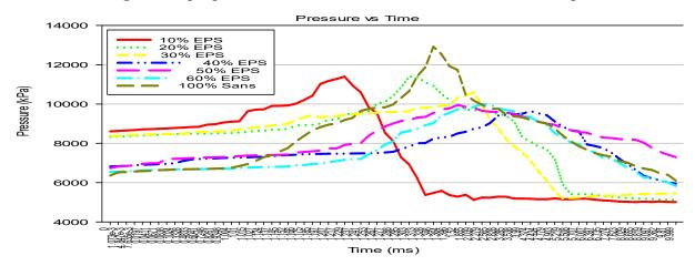
Fig.8. Overpressure versus time of EPS-sand mixtures and control sand sample
