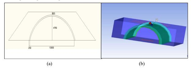
Fig.5. (a) Schematic diagram of the bunker (b) Location of gauge at ANSYS AUTODYN software
