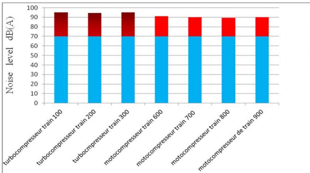
**Fig.9.** Histogram of comparison between the noise generated by the turbo-compressor and the noise generated by the Moto-compressor
