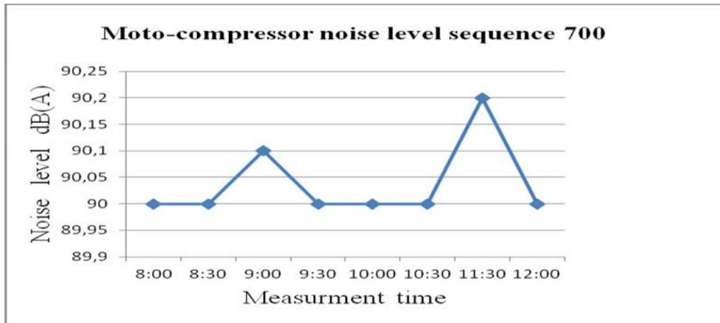
**Fig.8.** Noise level recorded in sequence 700
