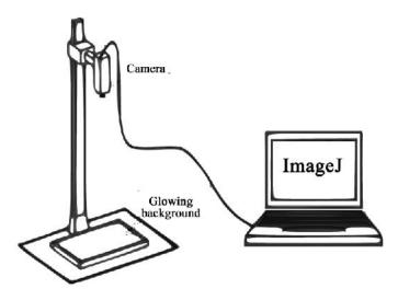
Fig. 2. Schematic diagram of the image acquisition setup
