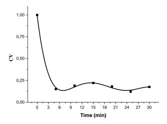
**Fig. 4.** Kinetics of the small particle of Starch with a concentration of 2% (w/w) in a Cubic mixer.
