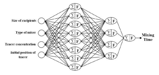
Fig. 6. Neural network used for the calculation of the mixing time
