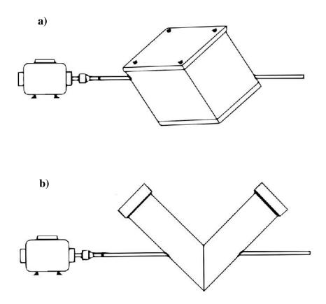
Fig. 1. Synoptic scheme of different blender: a) Cubic Blender, b) V- Blender.
