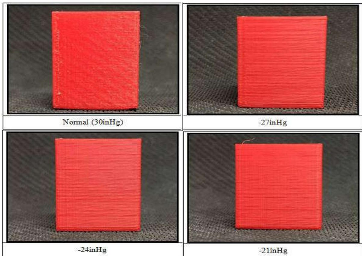
**Fig.8.** Plane of sample printed
