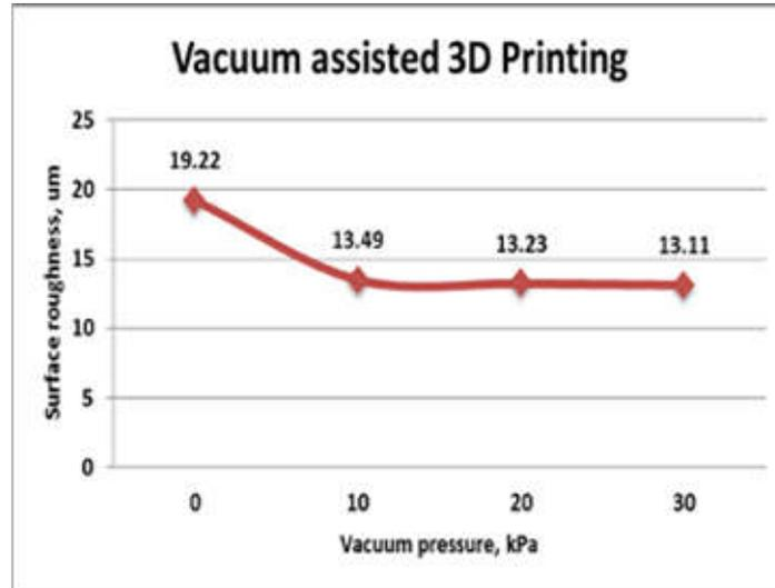
**Fig.9.** Comparison of surface finish value for normal vs integrated
