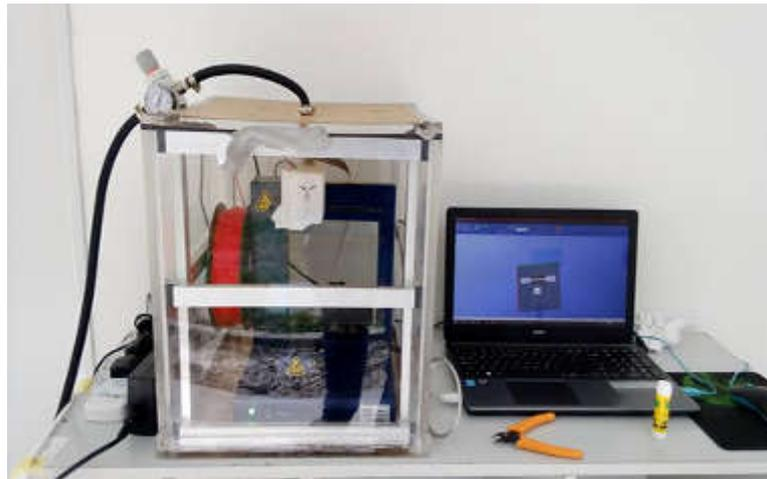
**Fig.4.** Vacuum technology integrated FDM Up Plus 2
