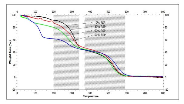
Fig.4. Thermo- gravimetric spectra of the polyurethane foams with varied amount of rice straw-based polyols (0%, 30%, 50% and 100%) replacement
