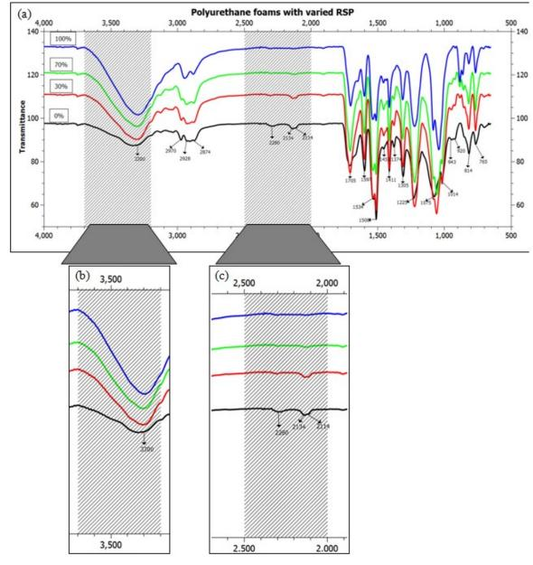
**Fig.3.** Over-all FTIR spectra of the PUF with varied amount of rice straw-based polyols (0%, 30%, 50% and 100%) replacement (b) in the region between 3100-3700 cm<sup>-1</sup> and between 2000-2500 cm<sup>-1</sup> (c).
