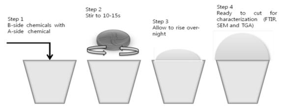
Fig.1. Procedure in synthesizing PU foam
