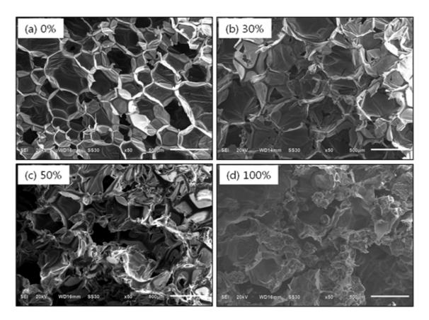
**Fig.2.** Scanning electron microscopy images of the produced polyurethane foams with a) 0% (petroleum-based polyols), b) 30%, c) 50% and d) 100% rice straw-based polyols replacement
