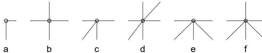
**Fig.1.** The number of elements in the nodes of a single-layered cylindrical grid shell: (a) two; (b), (c) four; (d), (f) six; (e) five. The circles show the nodal inserts
