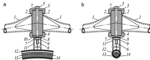
**Fig.4.** (a) and (b) are sections of the developed joint of the reinforced cylindrical grid shell:
