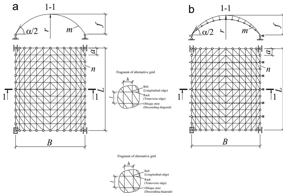
**Fig.2.** Plan and cross-section of the grid shell of the roof with geometric parameters: (a) without reinforcements (Scheme 1) and (b) with reinforcement of the diaphragms (Scheme 2)
