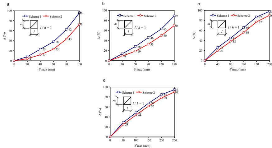
**Fig.5.** The effect of the introduction of joints with diaphragm elements on the percentage of depletion of the bearing capacity  $\Delta$  (%) and the maximum deflection  $\delta^z_{max}$  (mm) of single-layered cylindrical grid shells with square mesh size: (a) 1.8 m, (b) 2.38 m, (c) 3.01 m, (d) 3.6 m
