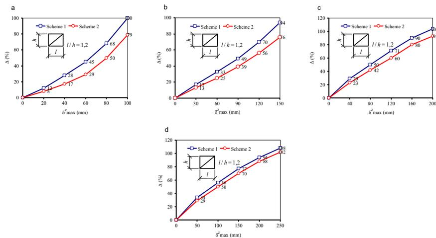
**Fig.6.** The effect of the introduction of joints with diaphragm elements on the percentage of depletion of the bearing capacity  $\Delta$  (%) and the maximum deflection  $\delta^z_{max}$  (mm) of single-layered cylindrical grid shells with rectangular mesh size: (a) 2.16x1.8 m, (b) 2.86x2.38 m, (c) 3.61x3.01 m, (d) 4.32x3.6 m
