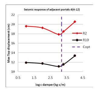
Fig.5. Peak response of two colliding intermediate steel frames for different records vs.
