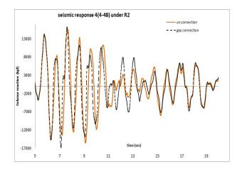
**Fig.2.** Free (-) and pounding-involved (--) Seismic response for collisions an intermediate moment steel frame with adjacent inverted-braced frame under record R2 of table 1.
