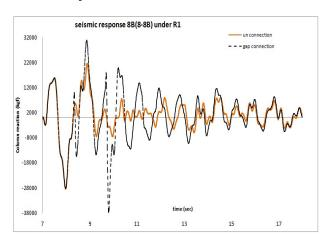
**Fig.3.** Free (-) and pounding-involved (--) Seismic response for collisions of an intermediate steel frame with a dual system of moment frame + invert bracing under record R1 of table 1.
