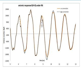
Fig.4. Free (-) and pounding-involved (--) Seismic response for collisions of two intermediate steel frames under record R6 in table 1
