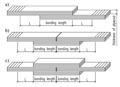
Fig.1. Types of adhesive joints
