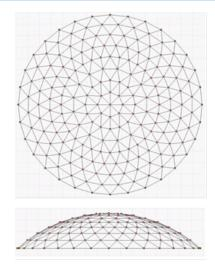
Fig.2. Plan and elevation of a spherical dome
