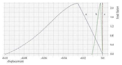
Fig.6. Variation of load factor with displacement at node n3 on ring 1 for C1
