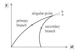
Fig.1. Nonlinear load path of a structure
