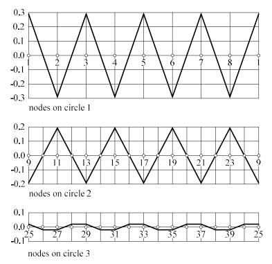
**Fig.4.** Vertical displacements in the normalized eigenvector for the singular state of C1 The computation of a singular point does not indicate whether the dome is unstable. In order to investigate the stability, the load path must be continued on the secondary branch. This topic is treated in [1]. It is shown that both load combinations have unstable singular points. The continuation also leads to the buckled shape of the dome.
