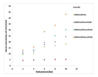
Fig.4. CO2/CH4 ideal selectivity in developed membranes as a function of pressure
