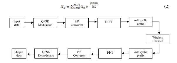
Fig.1. Diagram block conventional OFDM transceiver
