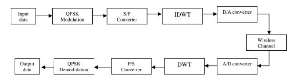
Fig.2. Block Diagram of Wavelet OFDM
