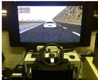
**Fig.1.** The driving simulator
