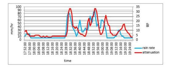
Fig.6. Combined rain attenuation and rainfall rate graph
