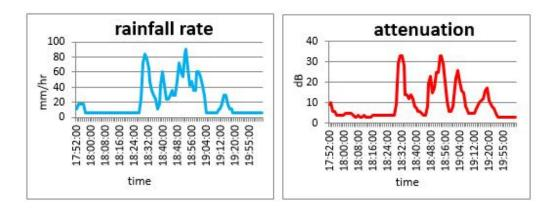
Fig.4. Rainfall rate on 19<sup>th</sup> June 2016Figure 5: Rain attenuation on 19<sup>th</sup> June 2016
