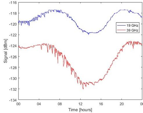
**Fig.2.** Example of 24h recorded signal level fluctuation due to satellite space motion which is the source for signal template (Prague, 6.1.2017)
