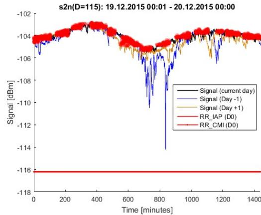
**Fig.4.** An example of polynomial template construction as one step of MY method (actual signal level data from December 2015)
