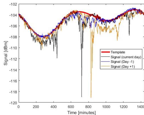
**Fig.7.** Constructed final template (red colour) after both polynomial and FFT/IFFT procedures applications (i.e. the MY method)
