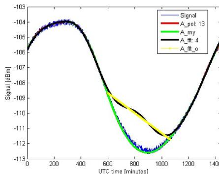
**Fig.3.** Example of good and worse template (FFT/IFFT method failed in this case)
