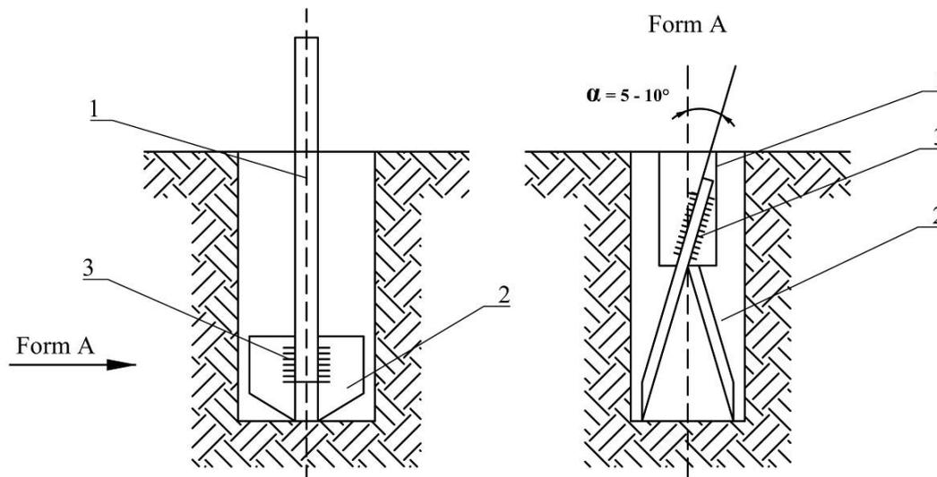
**Fig.2.** Dipping the equipment into the Soil
