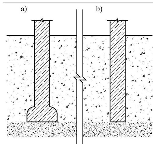
**Fig.1.** Scheme of bored piles
