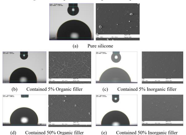
**Fig.5.** Image sequences of water droplets  $(5\mu L)$  of RTV's surface using organic and inorganic filler (Left) and Image of RTV's surface using scanning electron microscope (SEMs) (Right)
