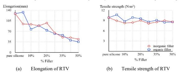
Fig.3. Comparison of (a) elongation (b) Tensile strength of RTV with organic and inorganic filler
