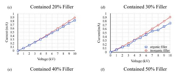
Fig.2. Comparison between the I-V characteristic of RTV using organic filler and inorganic filler in the same ratio
