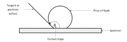
Fig.1. Measuring angle of contact
