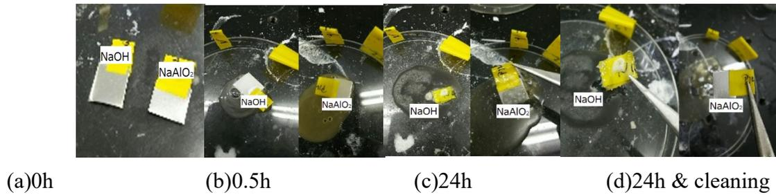
**Fig.3.** The difference in effect on aluminium at NaOH and NaAlO<sub>2</sub> (Left:NaOH,Right:NaAlO<sub>2</sub>)
