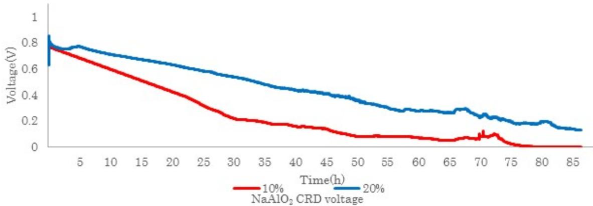
**Fig.11.** NaAlO<sub>2</sub> CRD voltage
