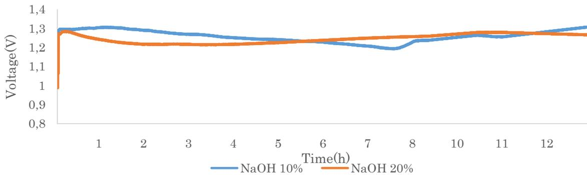
Fig.8. NaOH open circuit voltage
