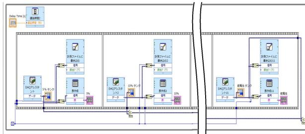
Fig.6. Labview program for measurement
