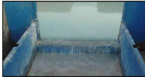
**Fig.3.** Spillway of thin wall tested (Model D1)
