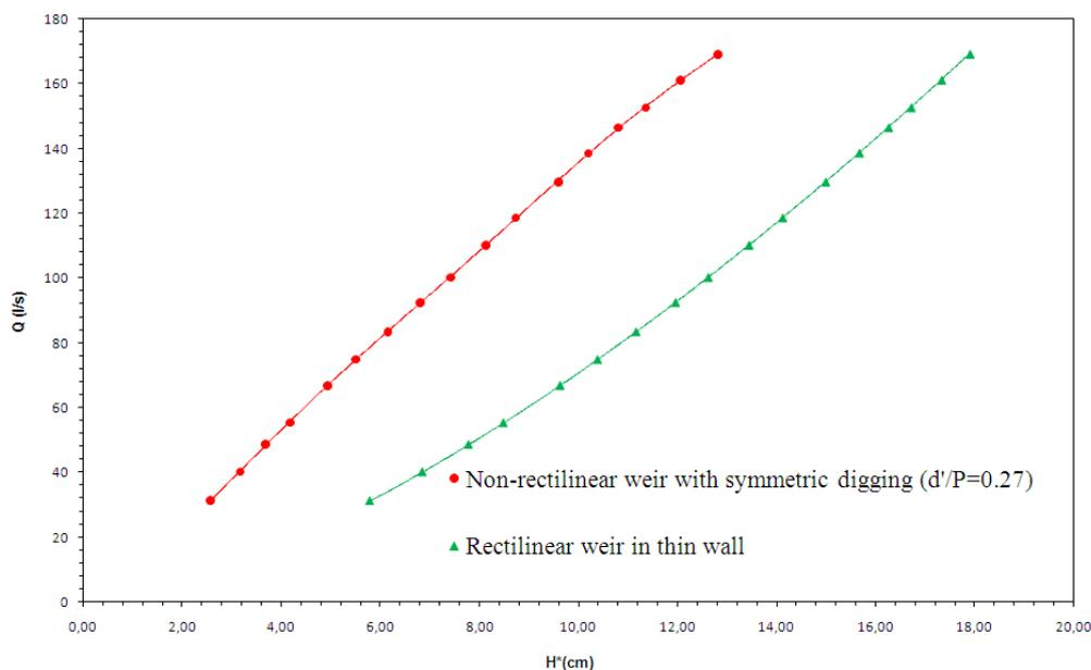
**Fig.6.** Flow curve of the spillway with symmetrical digging ( $d'/P = 0.27$ ) compared to that of the rectilinear spillway in thin wall
