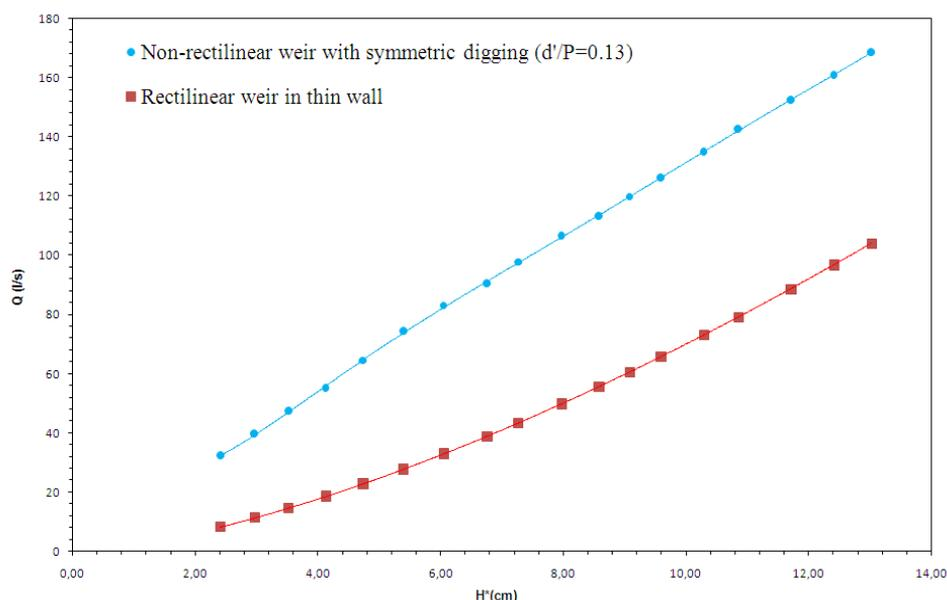
**Fig.5.** Flow curve of the spillway with symmetrical digging ( $d'/P = 0.13$ ) compared to that of the rectilinear spillway in thin wall
