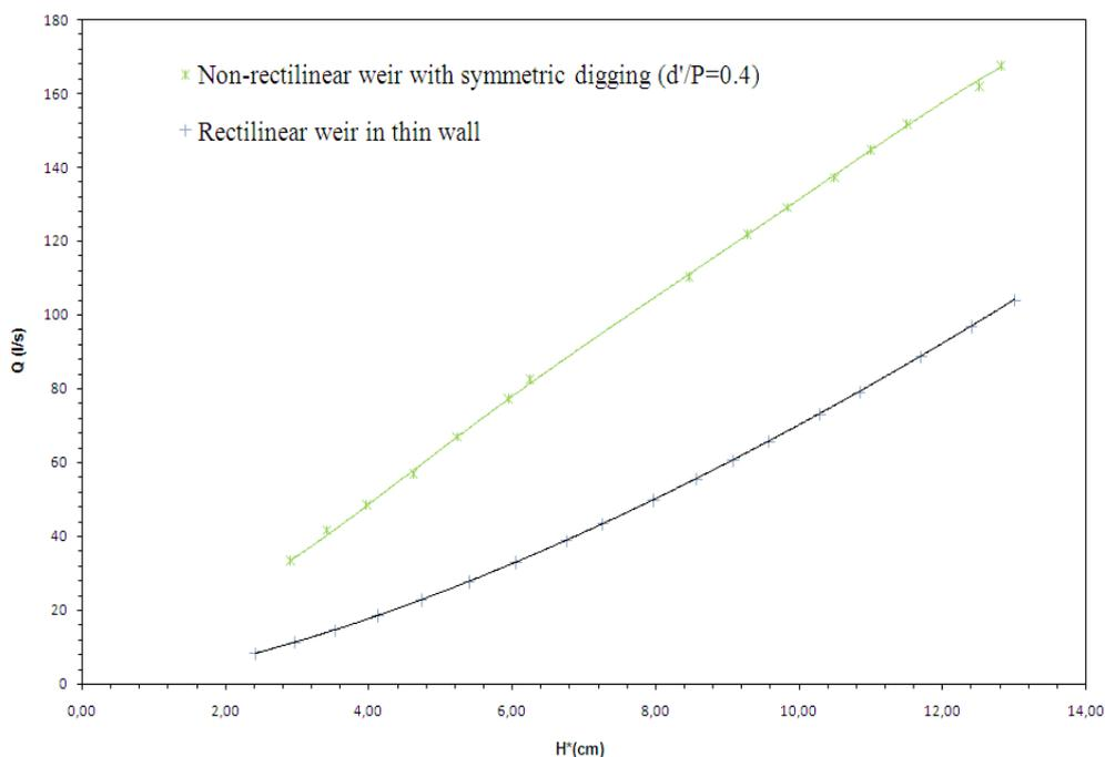
**Fig.7.** Flow curve of the spillway with symmetrical digging ( $d'/P = 0.4$ ) compared to that of the rectilinear spillway in thin wall
