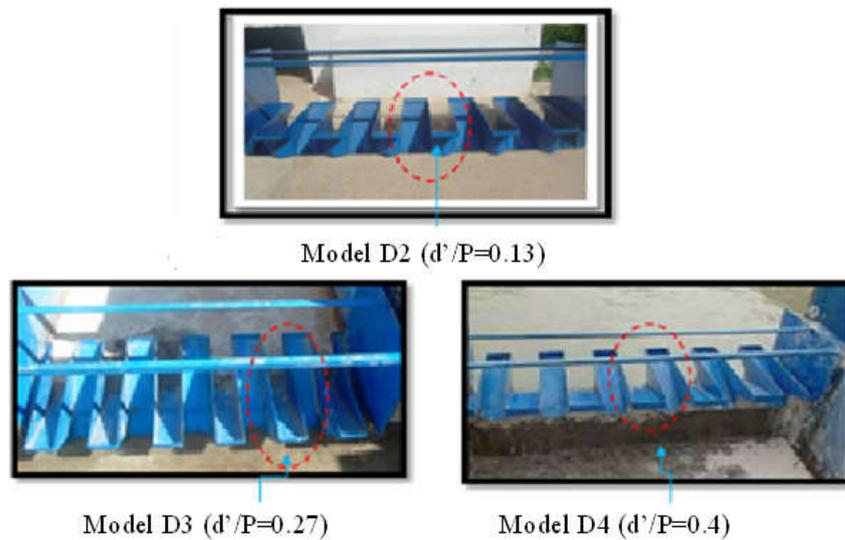
**Fig.4.** The tested models of spillways dug symmetrically
