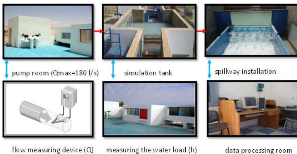
**Fig.2.** Experimental protocol (LAHE Laboratory – University of Biskra)
