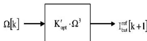
**Fig.6.** Reference Current According to Rotation Speed
