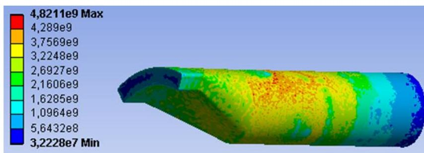
**Fig.14.** Variation of the equivalent stress with Von-Mises criterion
