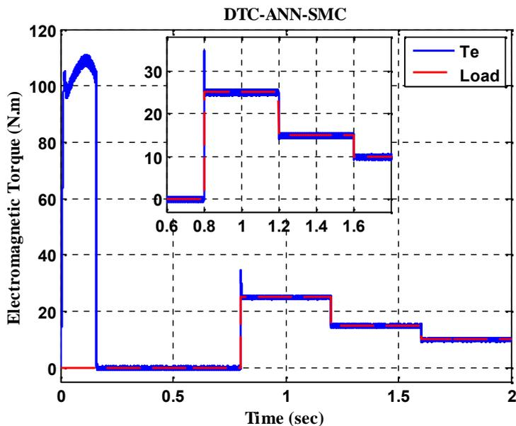
Fig.21. Torque response in DTC-ANN-SMC case
