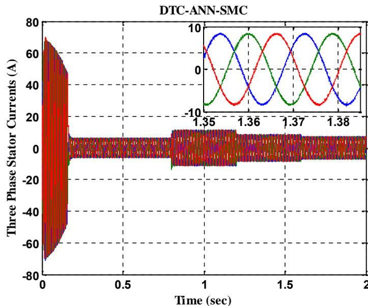
**Fig.30.** Three phase stator currents in DTC-ANN-SMC case
