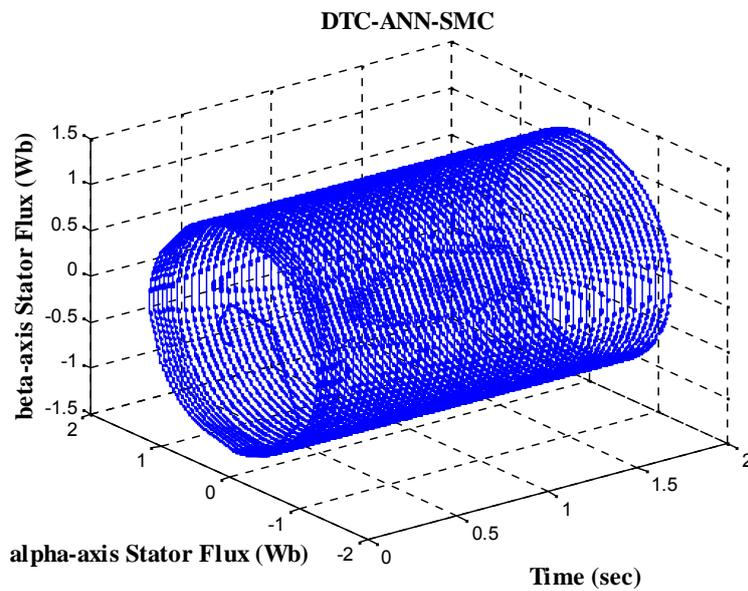
**Fig.28.** 3D representation of stator flux trajectory in DTC-ANN-SMC case
