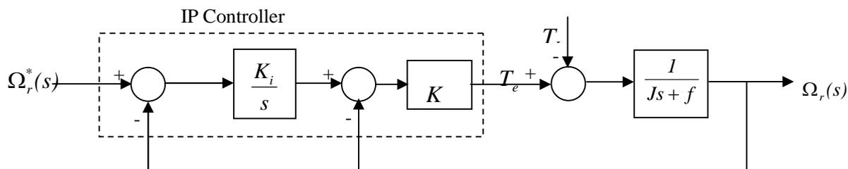
**Fig.4.** Speed control block diagram with IP controller
