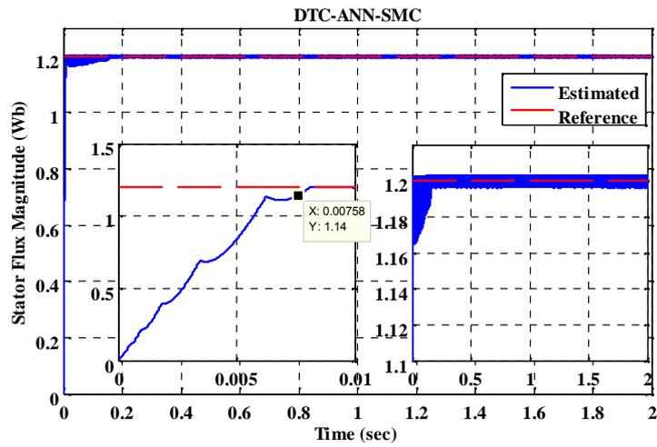
Fig.26. Stator flux magnitude in DTC-ANN-SMC case
