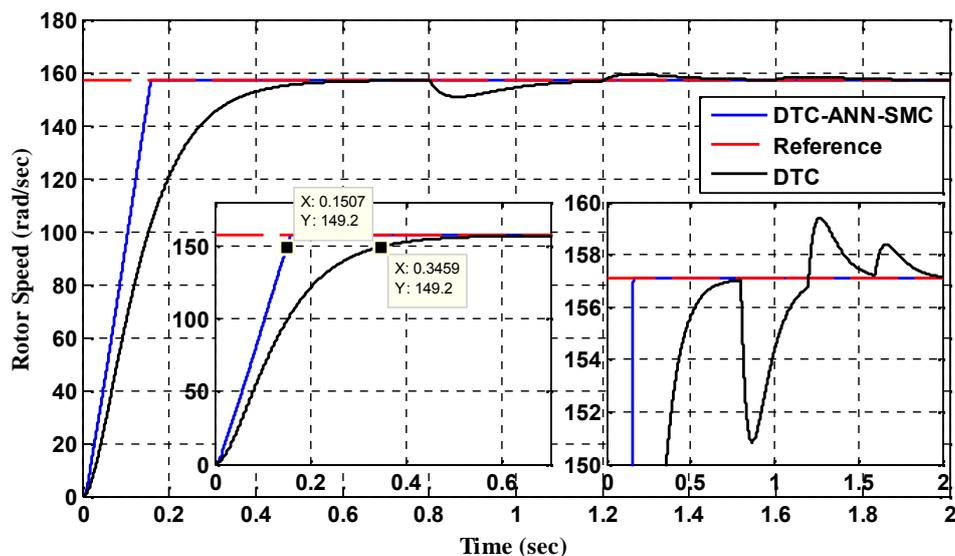
Fig.17. Comparison of speed response between DTC-IP and DTC-ANN-SMC
