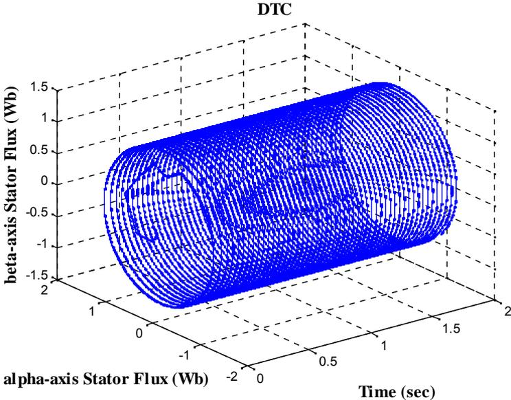
Fig.25. 3D representation of stator flux trajectory in DTC-IP case
