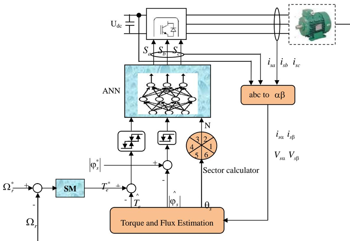
Fig.5. Proposed DTC diagram of the induction motor
