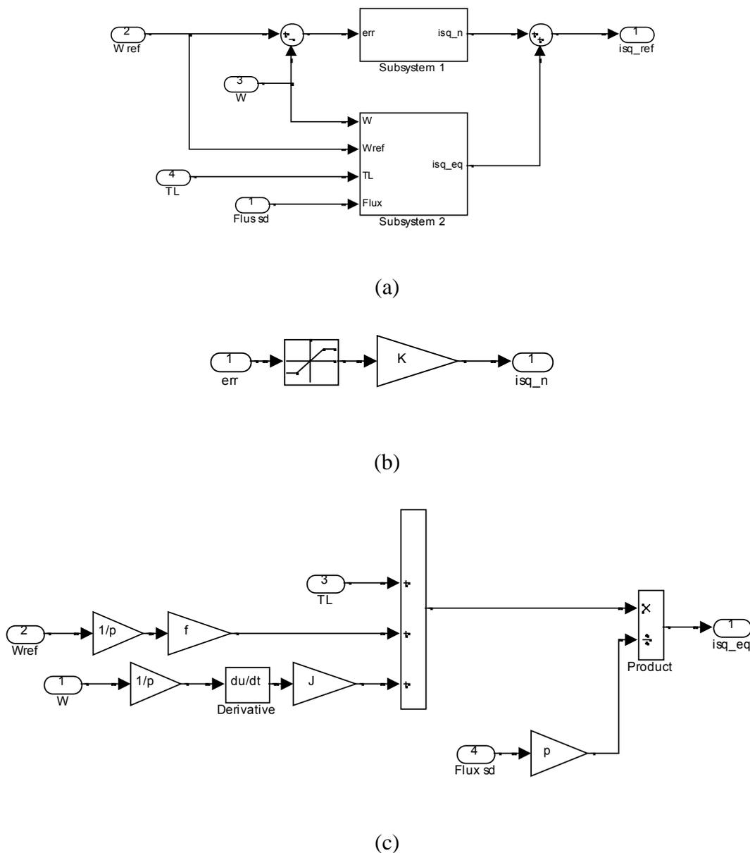
**Fig.6.** (a) Block diagram of speed control with SMC under Simulink, (b) Subsystem 1, (c) Subsystem 2
