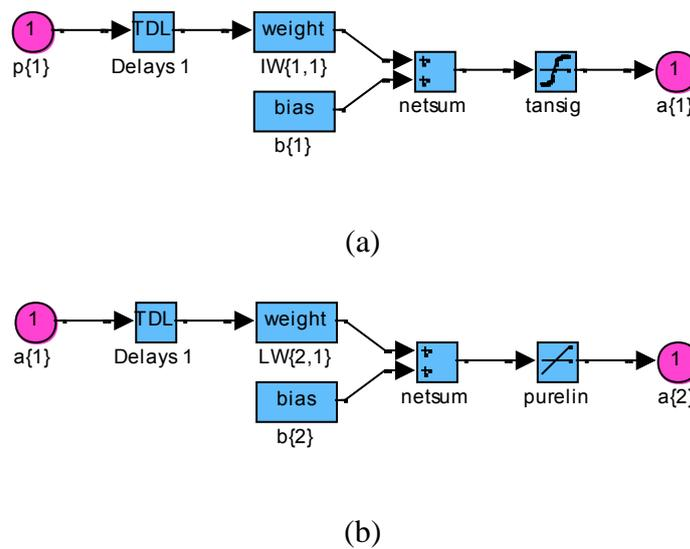
**Fig.13.** Details of ANN blocks in Fig. 12: (a) “Layer 1” and (b) “Layer 2”.
