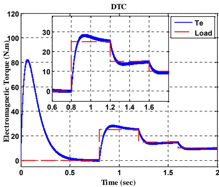
Fig.20. Torque response in DTC-IP case
