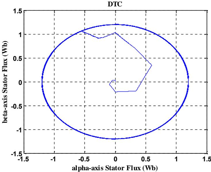
Fig.24. Stator flux trajectory in DTC-IP case
