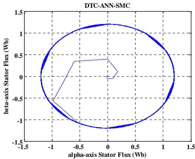
Fig.27. Stator flux trajectory in DTC-ANN-SMC case
