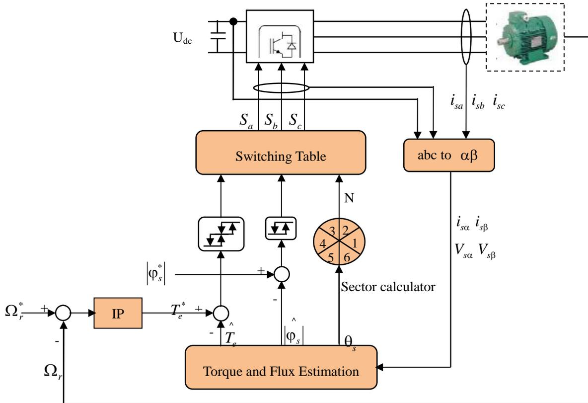
Fig.2. Classical DTC of an IM
