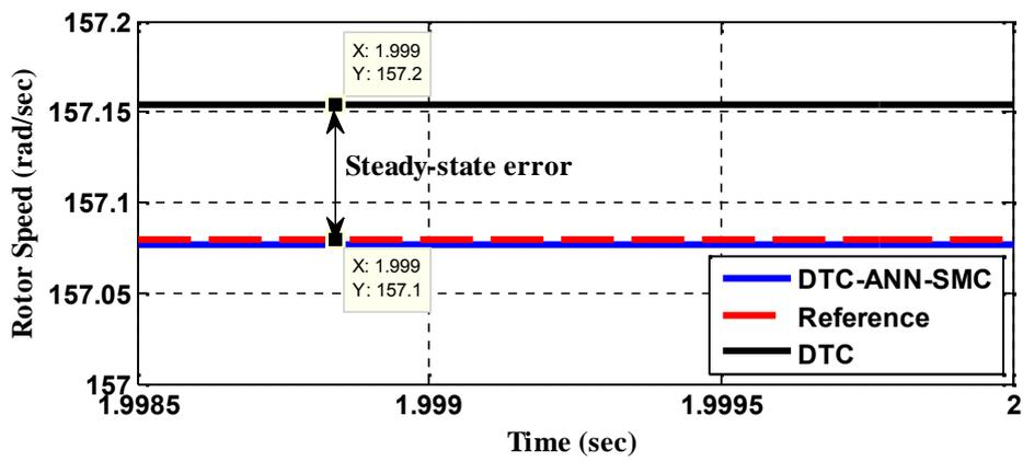
Fig.19. Comparison of steady-state error
