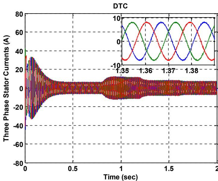
**Fig.29.** Three phase stator currents in DTC-IP case
