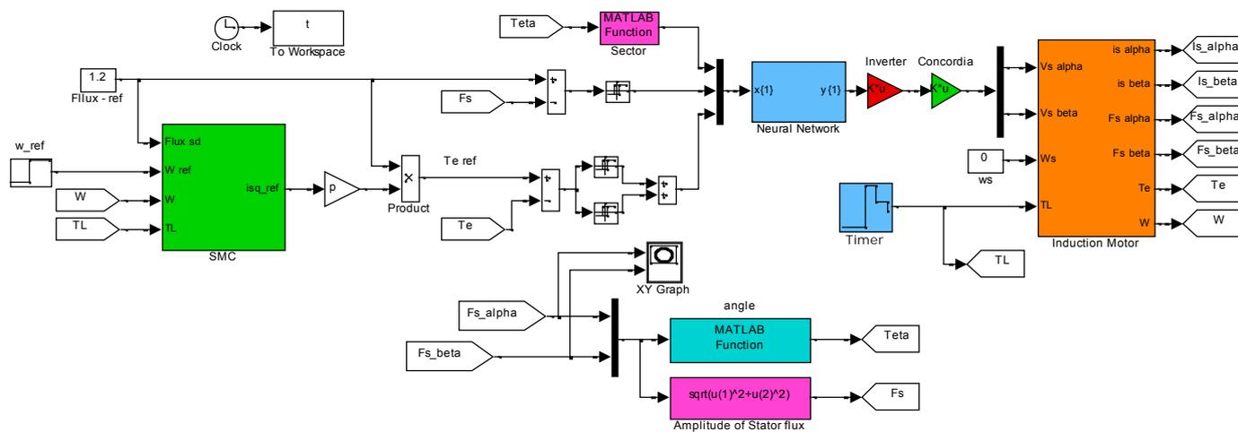
**Fig.7.** Block diagram of the proposed control under Simulink
