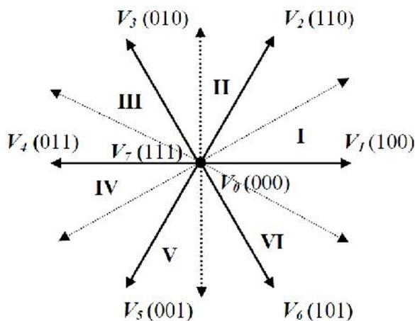
**Fig.3.** Stator flux vector locus and different possible switching vectors
