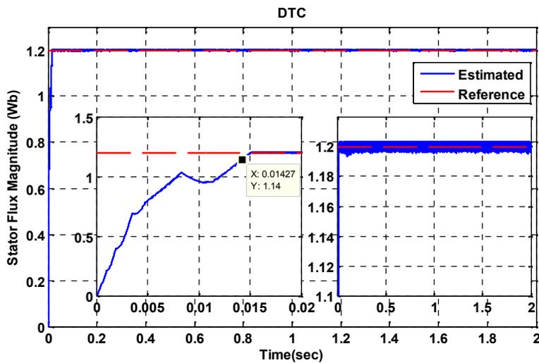
Fig.23. Stator flux magnitude in DTC-IP case
