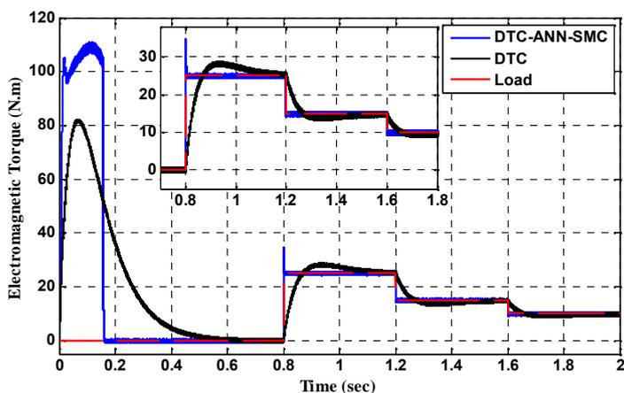
Fig.22. Comparison of torque response of DTC-IP and DTC-ANN-SMC
