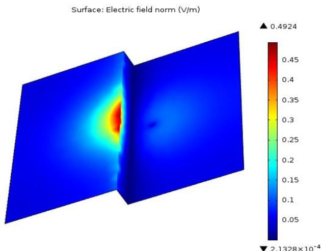
**Fig.9.b)** The computed electric field distribution on the discontinuous plane for a vertical lightning conductor
