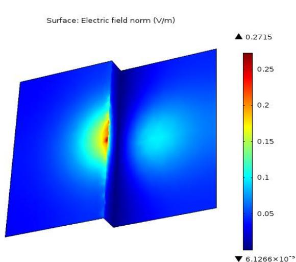
**Fig.11.a)** The computed electric field distribution on the discontinuous plane for a horizontal lightning conductor
