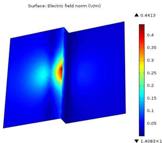
**Fig.7.a)** The computed electric field distribution on the discontinuous plane for a horizontal lightning conductor
