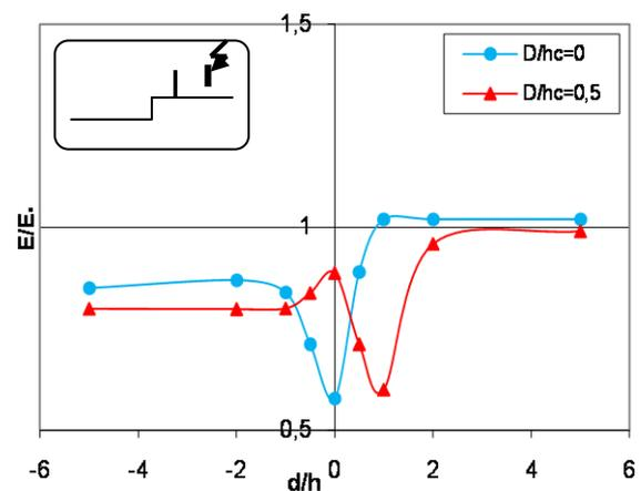
**Fig.4.b)** Electric field distribution with discontinuous conducting earth for a vertical lightning conductor
