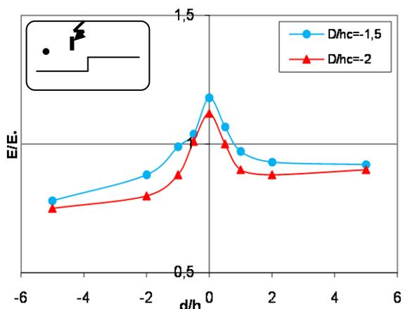
**Fig.8.a)** Electric field distribution with discontinuous conducting plane for a horizontal lightning rod
