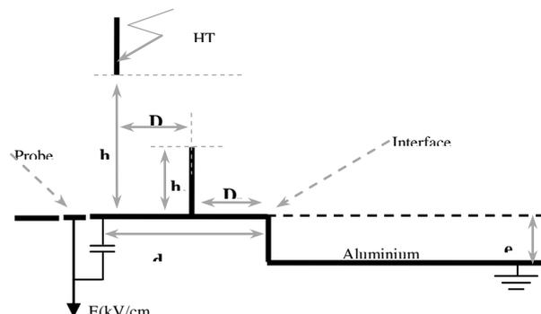
**Fig.1.b)** Configuration with discontinuous earth for a vertical lightning conductor
