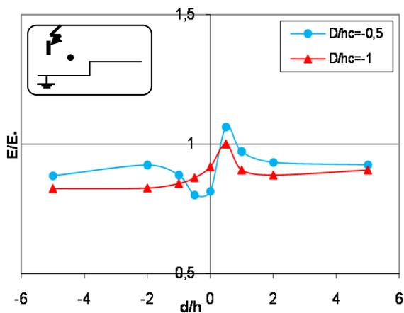
**Fig.10.a)** Electric field distribution with discontinuous conducting plane for a horizontal lightning rod
