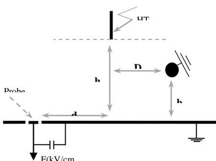
**Fig.2.a)** : configuration with homogeneous conducting earth for a horizontal lightning rod
