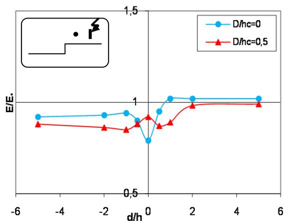
**Fig.4.a)** Electric field distribution with discontinuous conducting earth for a horizontal lightning conductor
