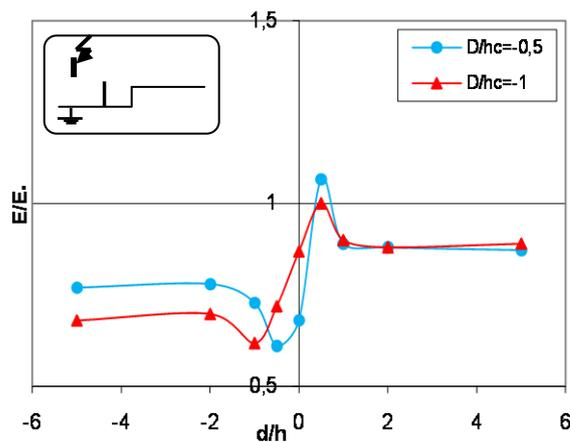
**Fig.10.b)** Electric field distribution with discontinuous conducting plane for a vertical lightning rod
