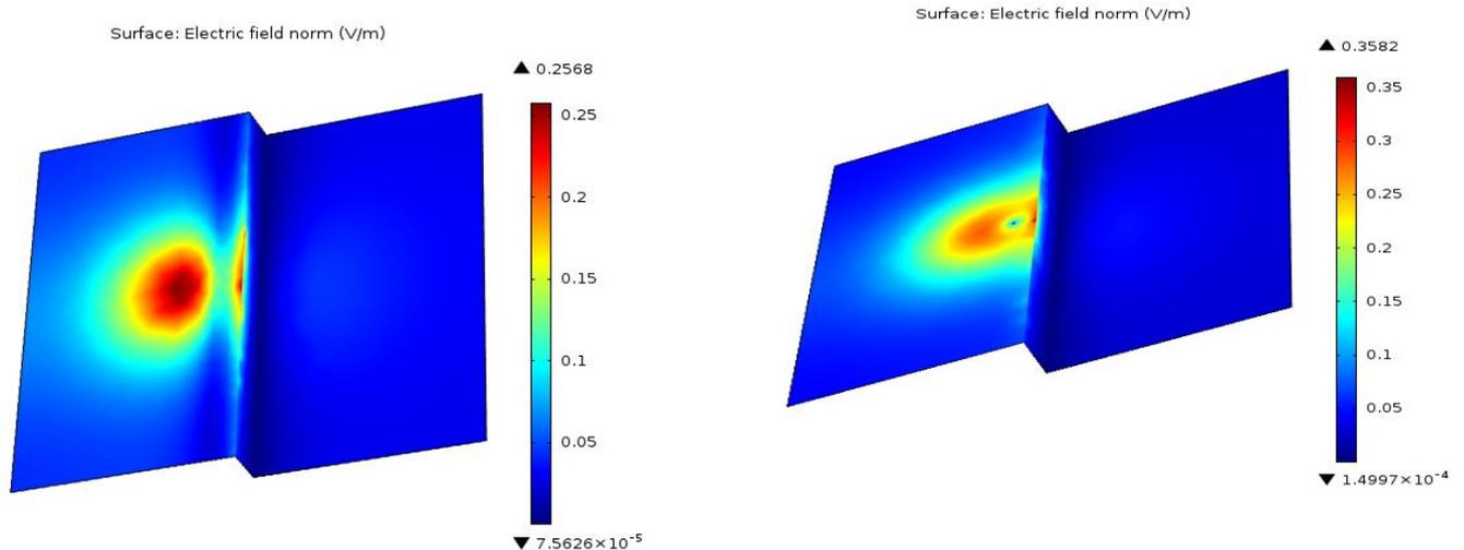
**Fig.5.a)** the computed electric field distribution on the discontinuous plane for a horizontal lightning conductor
