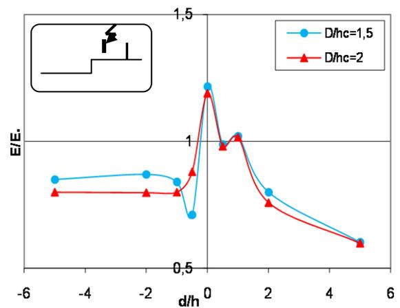
**Fig.6.b)** Electric field distribution with discontinuous conducting plane for a vertical lightning rod
