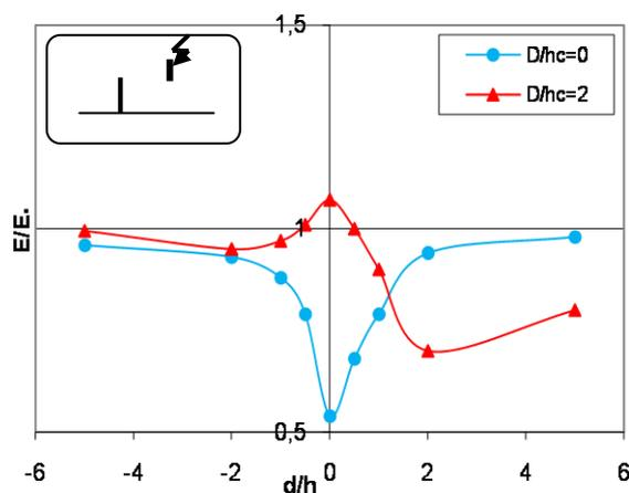
**Fig.3.b)** Electric field distribution with homogeneous conducting earth for a vertical lightning rod
