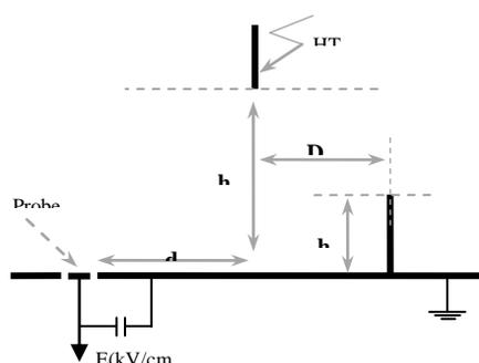
**Fig.2.b)** : configuration with homogeneous conducting earth for a vertical lightning rod
