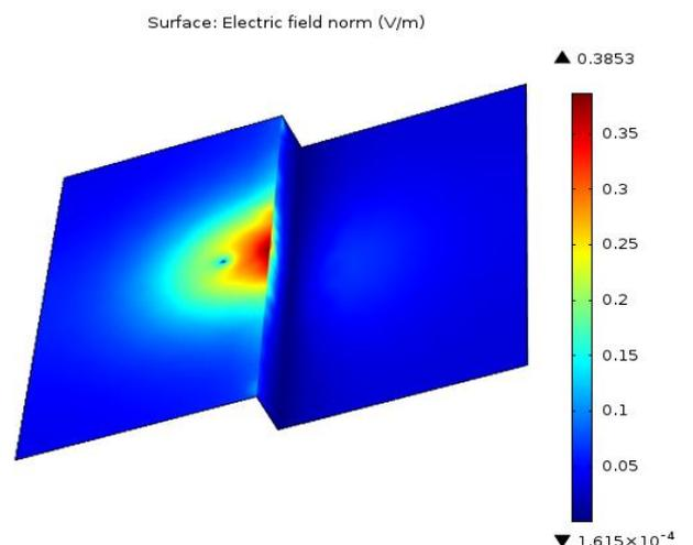
**Fig.7.b)** The computed electric field distribution on the discontinuous plane for a vertical lightning conductor
