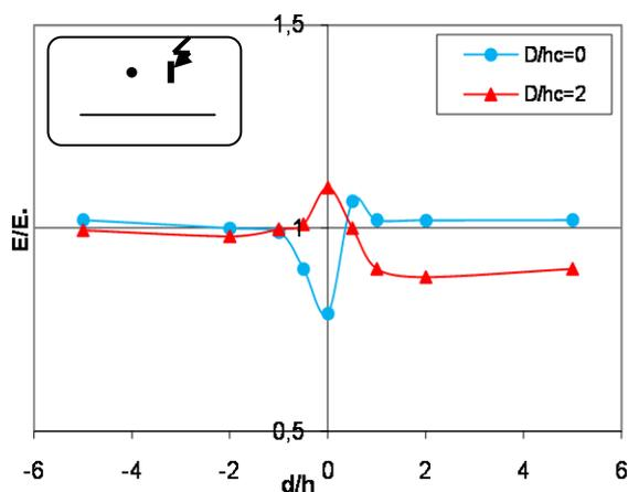
**Fig.3.a)** Electric field distribution with homogeneous conducting earth for a horizontal lightning rod
