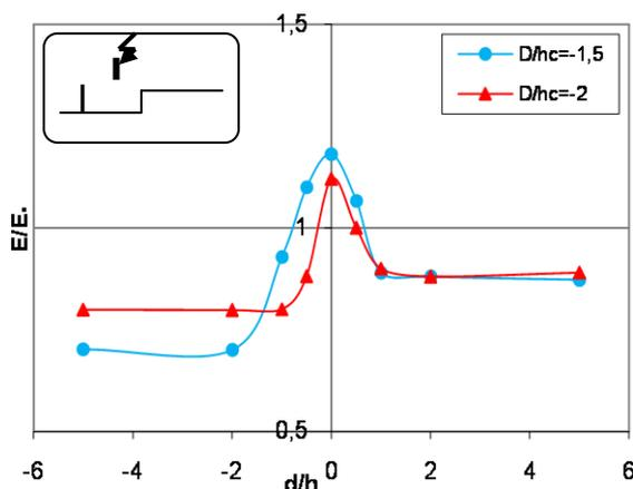
**Fig.8.b)** Electric field distribution with discontinuous conducting plane for a vertical lightning rod
