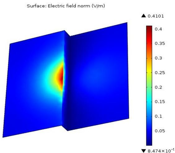
**Fig.9.a)** The computed electric field distribution on the discontinuous plane for a horizontal lightning conductor
