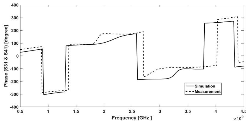
**Fig.6.** Phase difference phase S31–phase S41 of the dual proposed coupler
