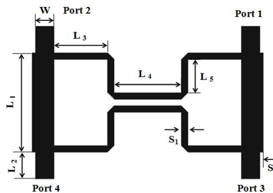
**Fig.3.** Geometry and dimension of the proposed coupler.
