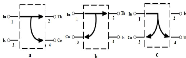
**Fig.1.** Three types of COD directional couplers with Input, through, isolation and coupled port
