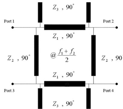
**Fig.2.** A novel dual-band proposed quadrature coupler with open-circuit stubs [4].
