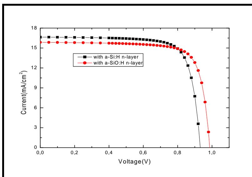
**Fig.3.** Simulated current-voltage characteristics of single junction a-Si:H solar cell structures.
