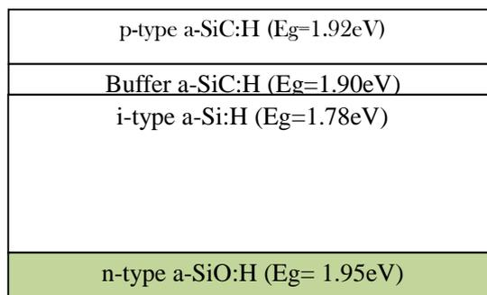
**Fig.1.** Design of a-Si:H p-i-n solar cell structure with n-type a-SiO:H layer
