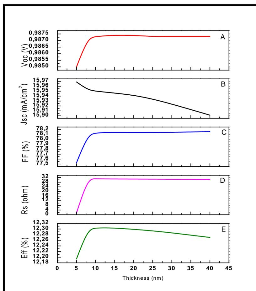
**Fig.2.** Variation of the parameters of a-Si:H solar cell as a function of a-SiO:H n-layer thickness, (A) Open circuit voltage, (B) short circuit current density, (C) Fill factor, (D) Serie resistance, (E) Efficiency.
