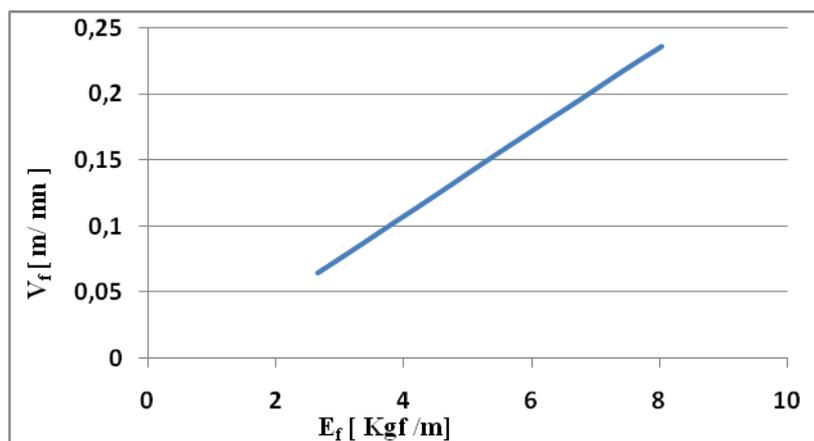
**Fig.6** The variation of the drilling speed
