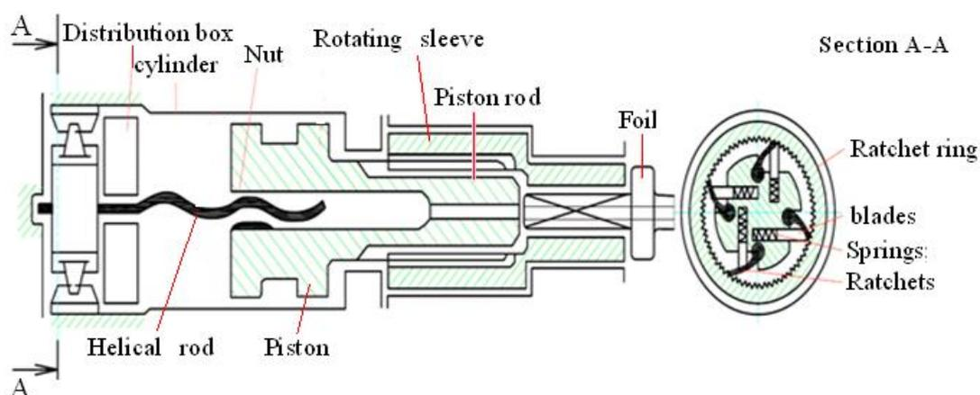
**Fig.2.** Longitudinal section of RH571- 4W drill Hammer [12]
