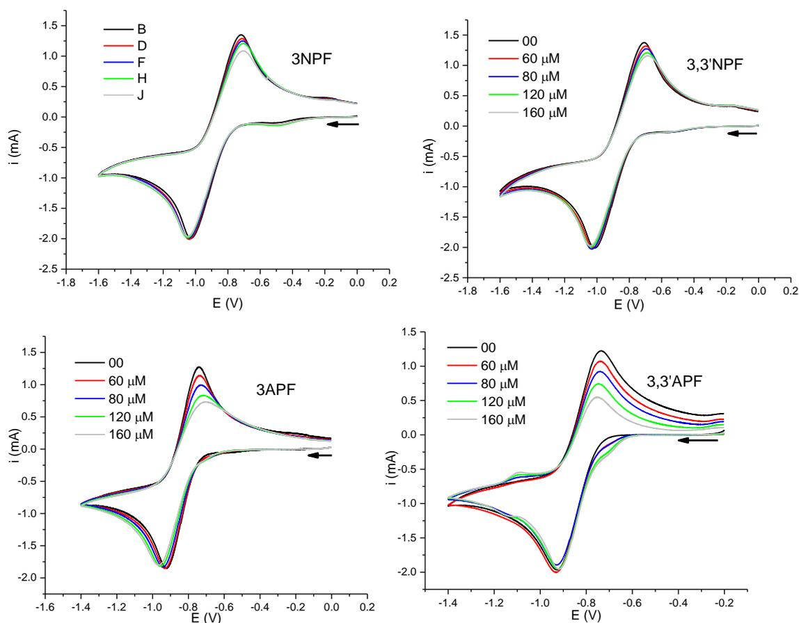
**Fig. 2.** Cyclic voltammograms of oxygen-saturated ACN/0.1 TBFB in the absence and presence of the test compounds at scan rate  $0.1 \text{ V}\cdot\text{s}^{-1}$
