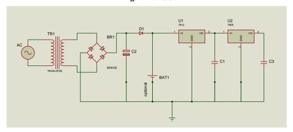
Fig.3. The PSU with a 12 V DC battery option
