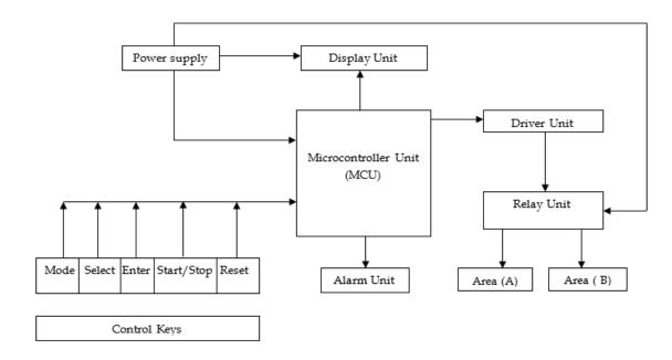
Fig. 1. The block diagram of the proposed UPDT switch
