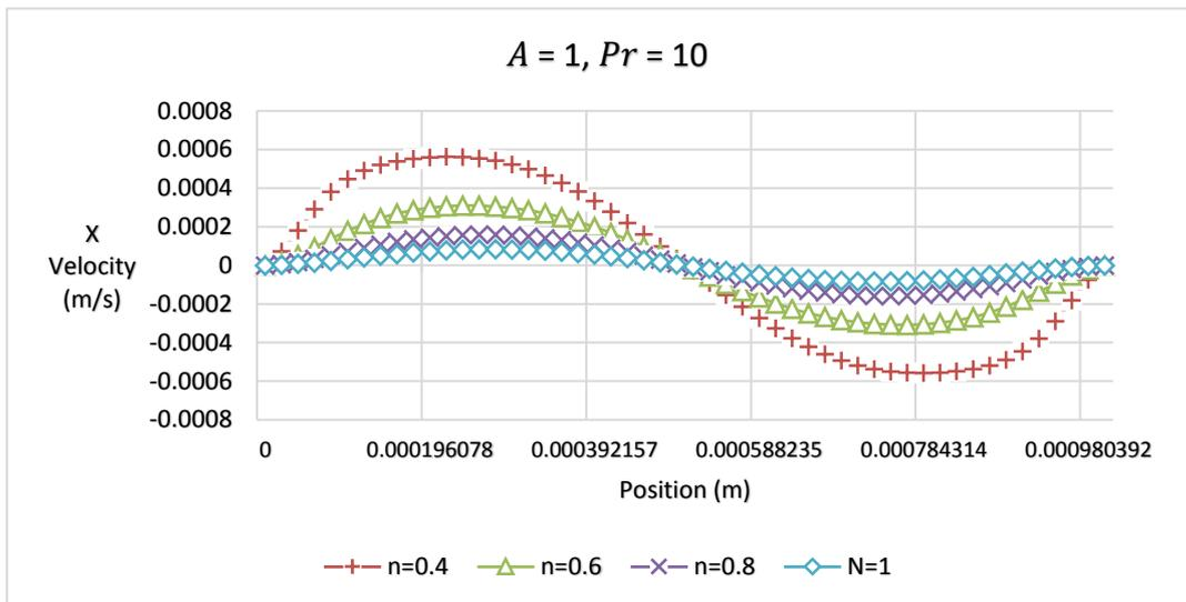
**Fig.10.** Effect of the fluid index "n" on the variation of the components of the velocity "u" as a function of X for Ra = 4000, E = 0.4, s = 0.01
