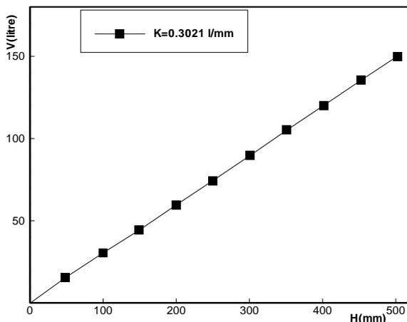
**Fig.5.** Calibration curve of the measuring tank
