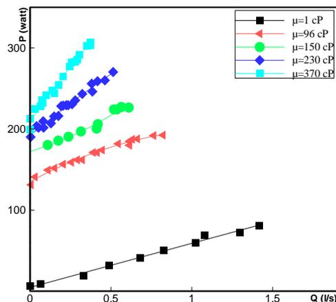
**Fig.16.** Power flow rate
