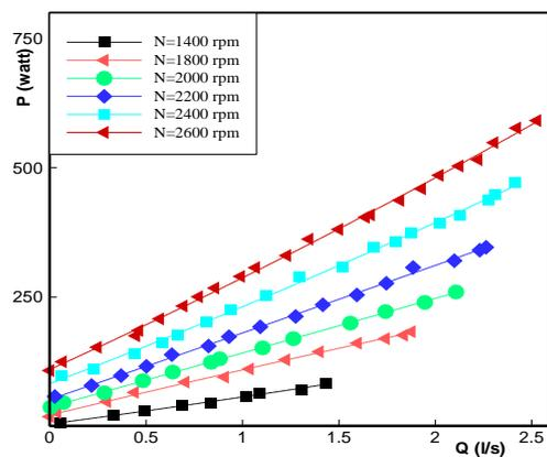
**Fig.9.** Power versus flow rate
