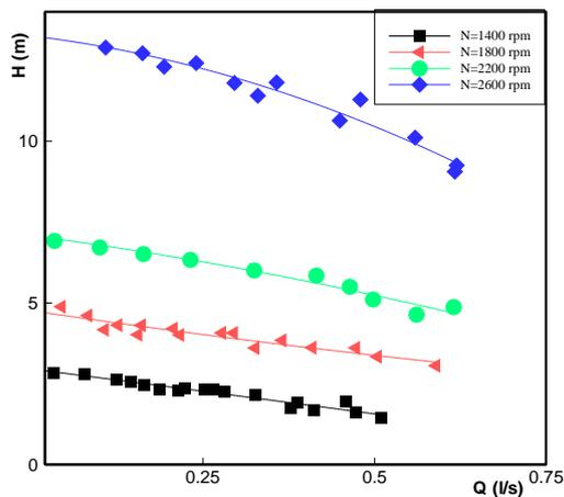
**Fig.10.** Head versus flow rate
