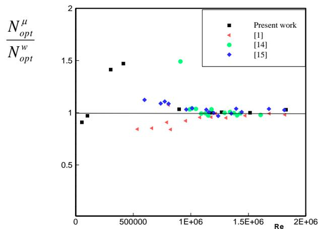
**Fig.20.** Ratio of the specific velocity as a function of Re at the points of best efficiency for viscous fluids and water
