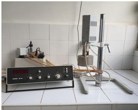
**Fig.2.** Experimental rig of Viscometer
