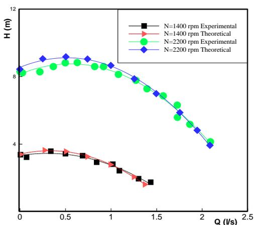
**Fig.6.** Head versus flow rate ( $\mu=10^{-3}$  Pa.s)
