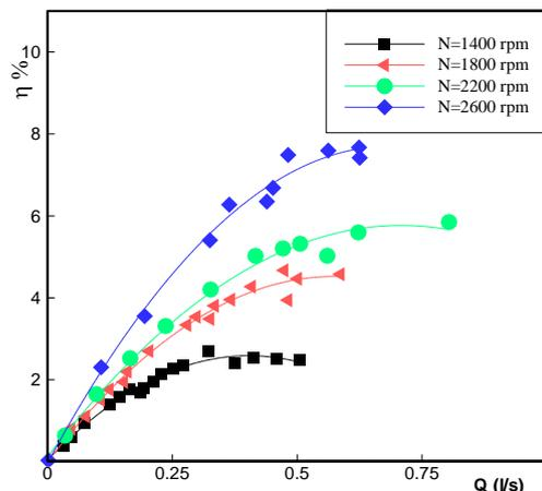
**Fig.12.** Efficiency versus of flow rate ( $\mu= 230.10^{-3}$  Pa.s)
