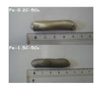
Fig.1. The annealed alloys before cutting
