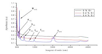
**Fig.2.** Absorption spectrum of Er+3 in the glass (60Sb2O3-20Na2O-20WO3)
